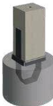
Column Base Connection
