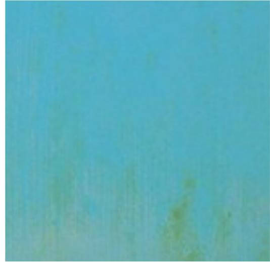
**FIGURE 13.** Color loss and overall deterioration of paint film on fresh masonry.
