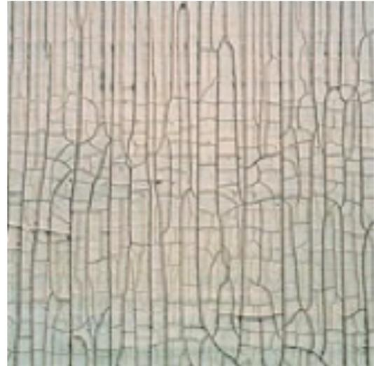
**FIGURE 1. Patterned cracking in the surface of the paint film resembling the regular scales of an alligator.**
