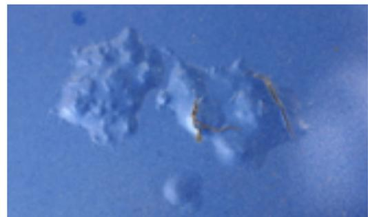
**FIGURE 2. Bubbles resulting from localized loss of adhesion and lifting of the paint film from the underlying surface.**
