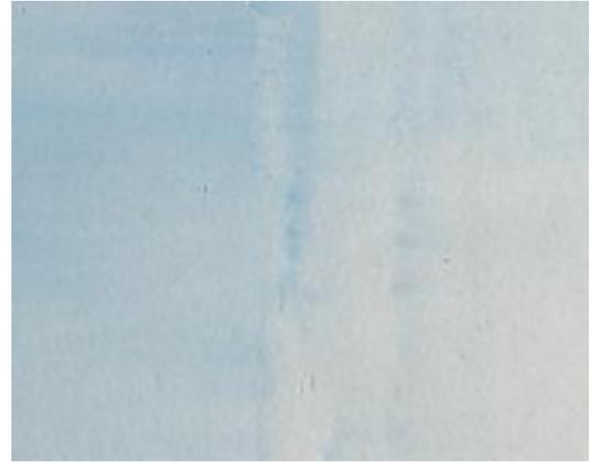
**FIGURE 11. Appearance of a denser color or higher gloss where wet and dry layers overlap during paint application.**
